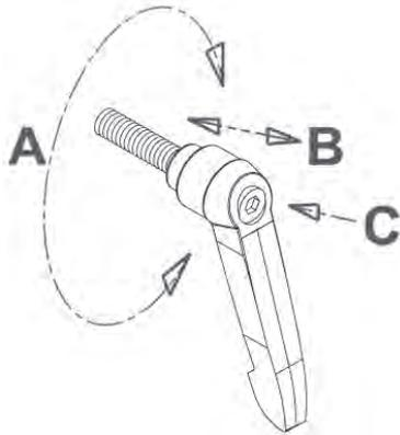
**NOTE:** Insert the ratchet handle through the unthreaded side of the articulated swing arm and tighten. Going through threaded side first will not allow the arm to tighten properly
