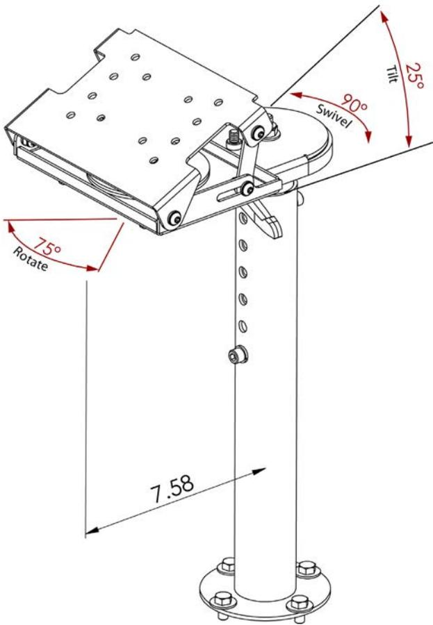
Adjust the height of the tube assembly as needed by removing the (2) 5/16-18 socket head cap screws with the provided 1/4" hex key. Re-tighten once desired height is reached.
