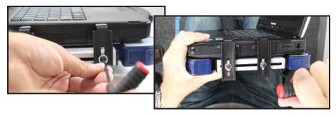
4.2) Using the New Side Clamps, install one New Side Clamp into each the slots that the Original Side Clamps were in previously. Tighten the screws. Ensure that all Side Clamps slide over the top edge of your laptop before moving to step 5.
